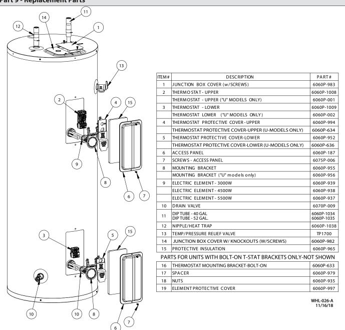
Figure 8 - Replacement Parts - Staged Operation
