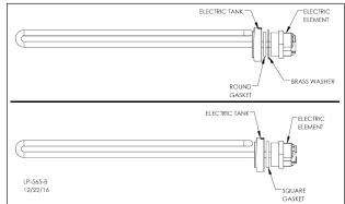
Figure 7 - Heating Element Detail
